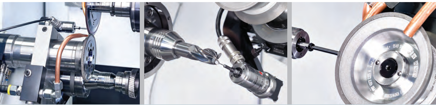
Dressing attachment that saddles the workpiece axis (A-axis)
